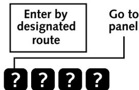
Enter by the designated entry route. The entry tone starts. Go to the control panel and key in your four digit user code (or press OFF on your 525r remote setting device). The system switches off.
